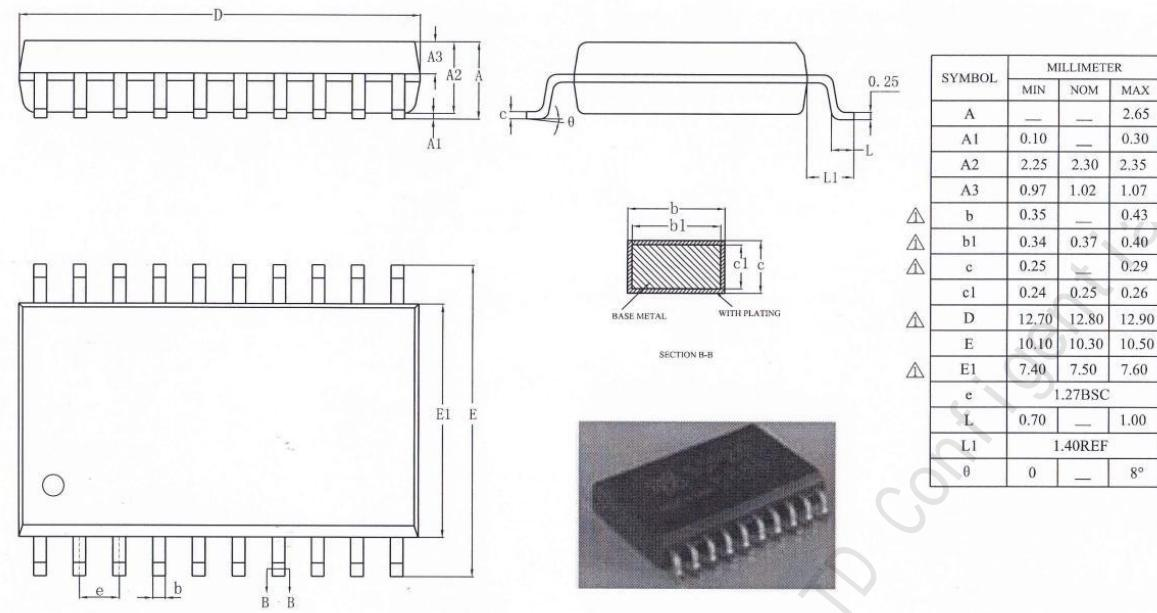
Figure 1-13 Encapsulation POD of SOP20
