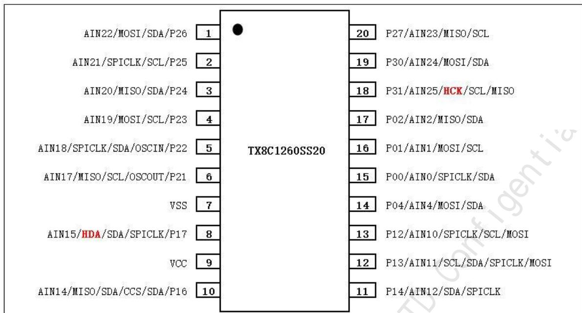
Figure 1-4 Pin of TX8C1260SS20 (SSOP20)
