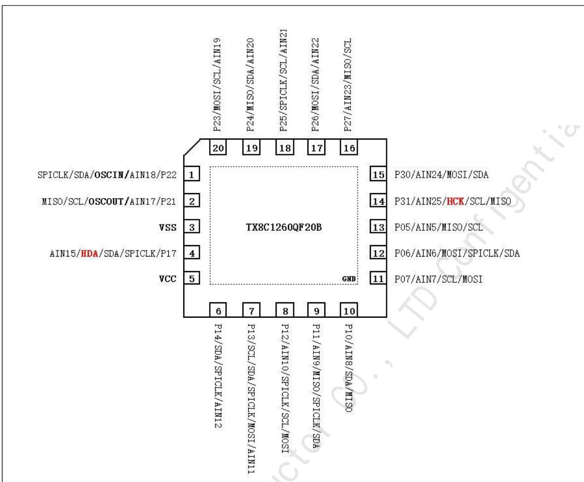
Figure 1-3 Pin of TX8C1260QF20B (QFN20)
