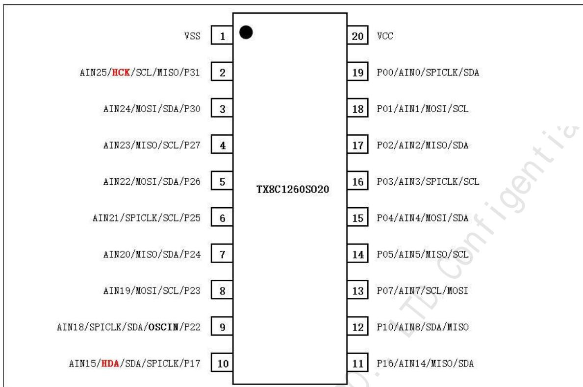
Figure 1-6 Pin of TX8C1260S020 (SOP20)
