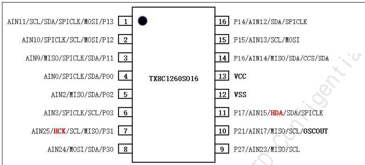
Figure 1-8 Pin of TX8C1260S016 (SOP16)
