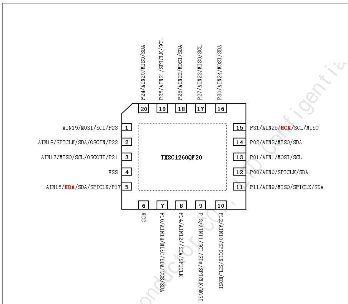
Figure 1-2 Pin of TX8C1260QF20 (QFN20)
