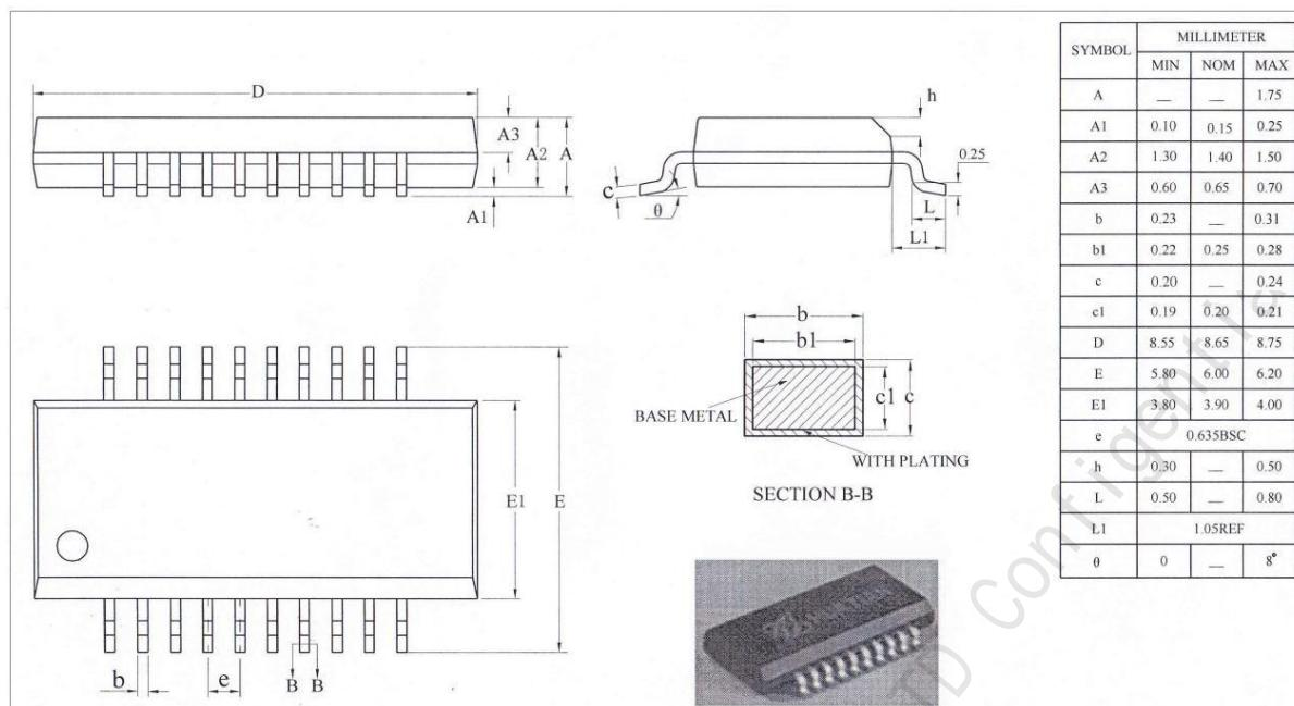
Figure 1-11 Encapsulation POD of SSOP20
