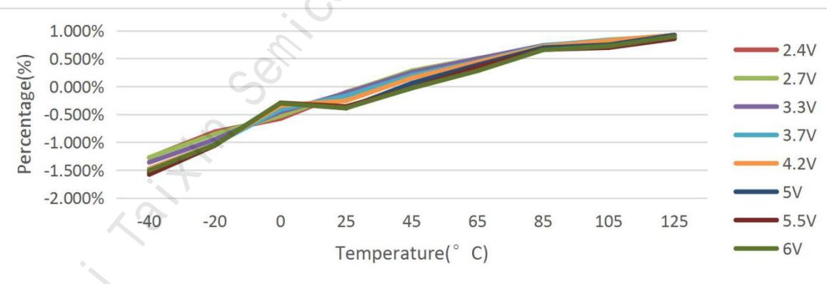
Figure 2-3 HIRC deviation under all voltage and all temperature
