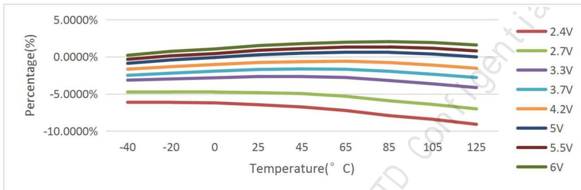
Figure 2-4 LIRC deviation under all voltage and all temperature
