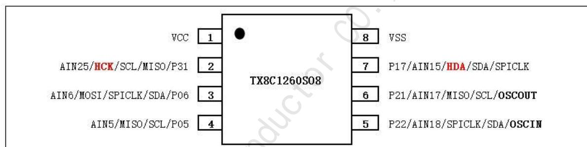
Figure 1-5 Pin of TX8C1260S08 (SOP8)
