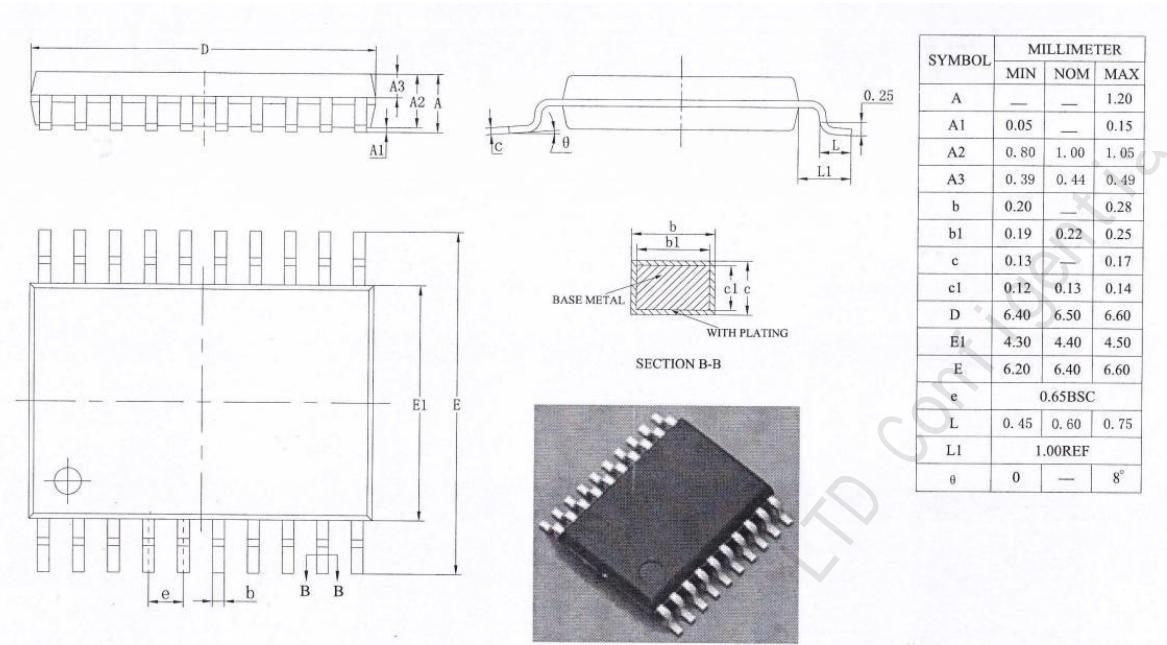
Figure 1-9 Encapsulation POD of TSSOP20
