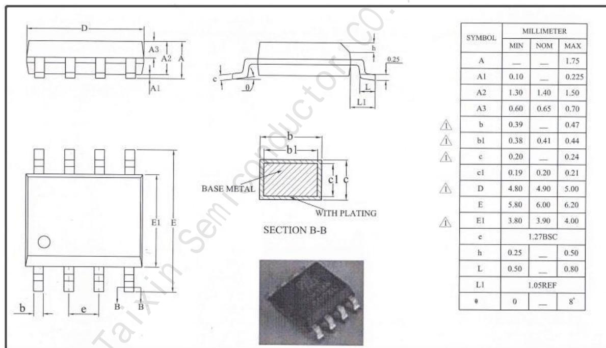
Figure 1-12 Encapsulation POD of SOP8
